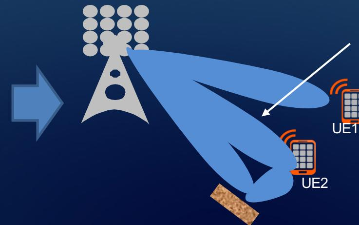
Finding the best combination of users and optimize beam and perform zero forcing in order to maximize spectrum efficiency
