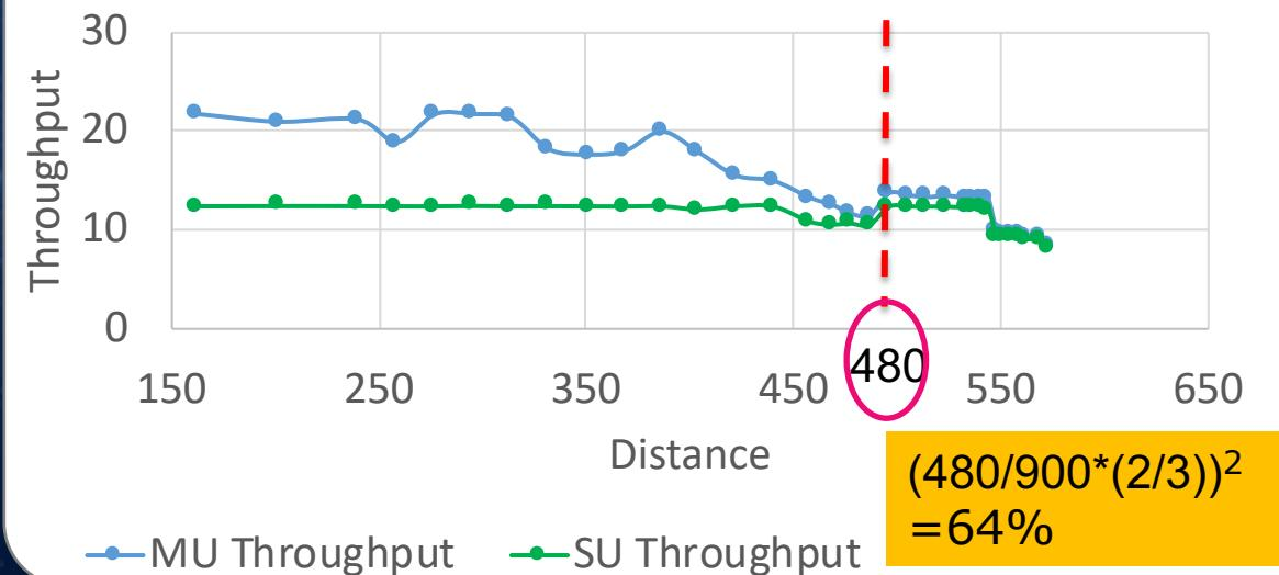
For 900M ISD, Vertical TRX Can Provide Vertical UE Paired in >64% Cell Area
