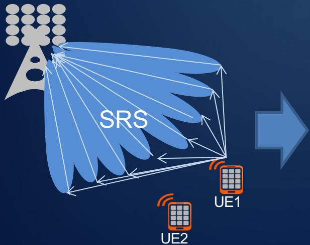
**Receives SRS on different beams**
