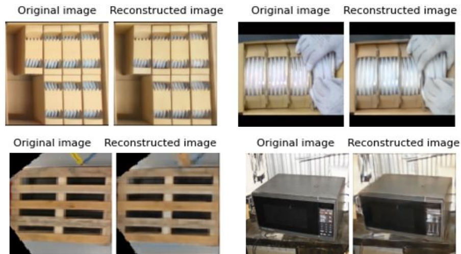
5.1. Figure - The Vanilla autoencoder method well-reconstructed images of the product (first), even if it contained anomalies (second), as well as images completely unrelated to the product (third, fourth).
