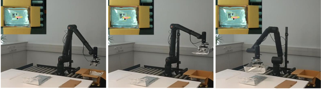
1.1. Figure - Images of a rudimentary version of the Unpacking Machine in work. It sorts the products based on its camera view, which is illustrated on the upper left side of the images.
