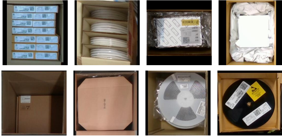
5.3. Figure - Examples for false positive detections, with unique characteristics. (1. is from stacked boxes, 2. is from side reels, 3. and 4. are from pizza boxes and 5. and 6 are from reels.)
