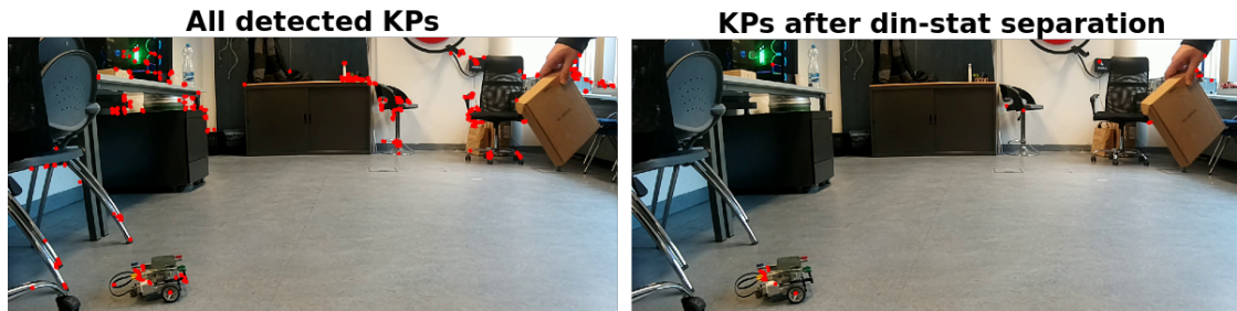
Figure 5.4: Operation of din-stat algorithm in presence of multiple dynamic objects.
