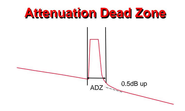
The distance of the Attenuation Deadzone is from the start of a reflective event until <u>0.5dB up from the backscatter</u> <u>level</u> after the reflection.
