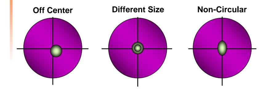
All fibers are allowed a certain tolerance in the core/cladding geometry. This can cause light loss at joints between fibers.
