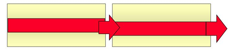
Off-center core in second fiber does not receive all the light from the first fiber. The amount of light lost is the Splice Loss.
