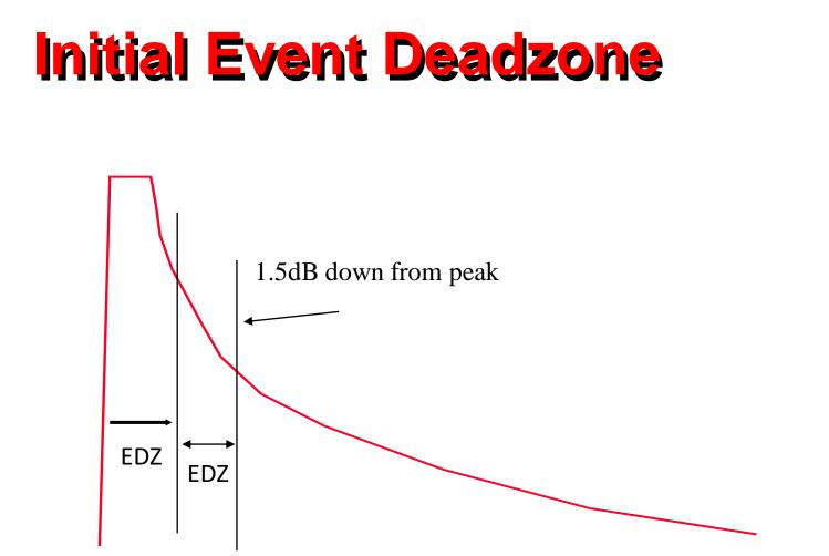
An OTDR's Initial Event Deadzone will have this appearance without a fiber connected to the OTDR.
