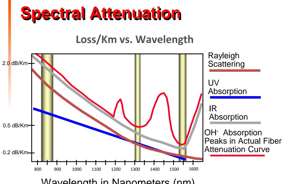
Wavelength in Nanometers (nm)
