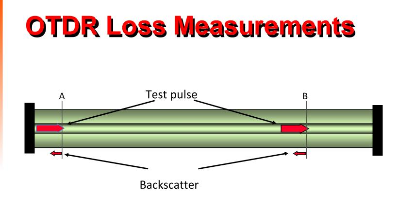
Backscatter is directly related to the level of light in the test pulse. As the level of light in the pulse width decreases with distance, so does the backscatter it produces.
