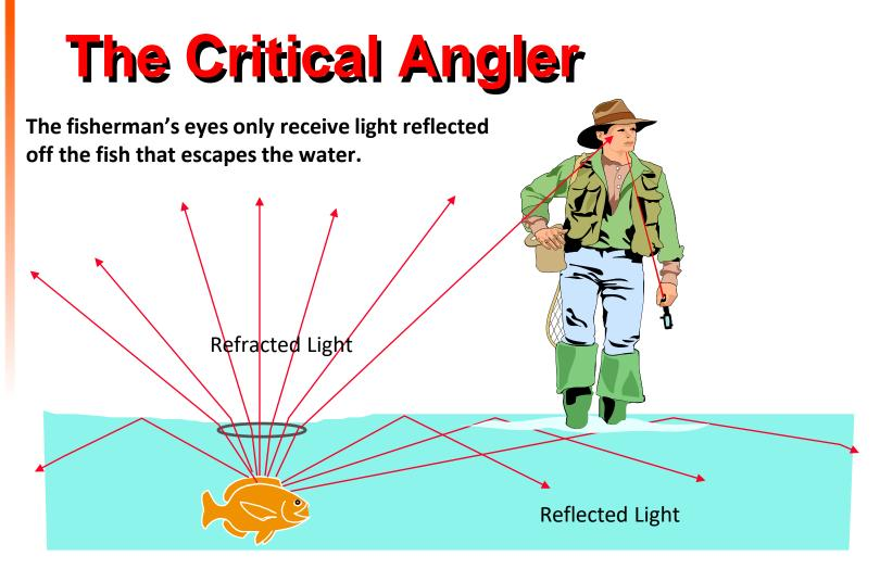
Light rays reflecting off the fish that strike the surface of the water at an angle outside that defined by the circle do not escape but are reflected back into the water.
