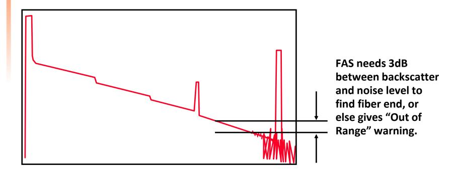
**REMEDY:** Select larger Pulse Width to increase Dynamic Range and/or set "End Detect Threshold" in FAS Setup to lower value.
