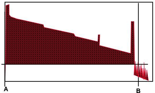
ORL is looked at from the transmitter's point of view. It is the total power returned to the transmitter from the fiber link and is typically expressed in dB. It includes the total Backscatter and all Reflections.
