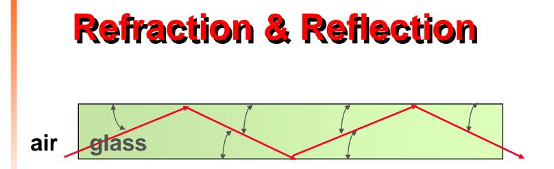
As long as the light ray stays at the Critical Angle or less as it hits the air-glass interface, it will remain in the fiber until it reaches the other end.
