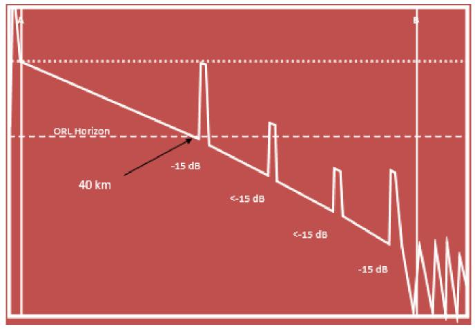
Reflections returning from farther than 40km will have not effect on the stability of the transmitter. Accurate ORL measurements do not require measuring to the end of a 150 km link. Only the first 40 km matter.
