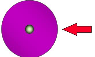
Singlemode fiber has a smaller core relative to the cladding diameter. 8 - 9 um is a typical core size centered in a cladding of 125 um.
