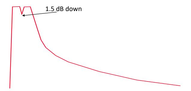
However, should the OTDR display the trace above when connected to a fiber at the patch panel, it can easily be seen that there are two events. The first is at the OTDR, the second is where the fiber is broken.
