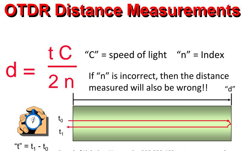
Speed of Light in a Vacuum is: 299,792,460 meters per second. Speed of Light in a Vacuum is: 186,287.5 miles per second.
