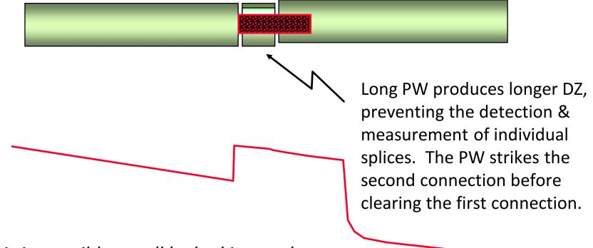
It is impossible to tell by looking at the trace which splice is causing the high loss.
