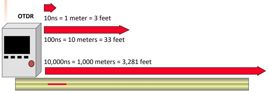
Only one test pulse is allowed in the fiber at any time.
