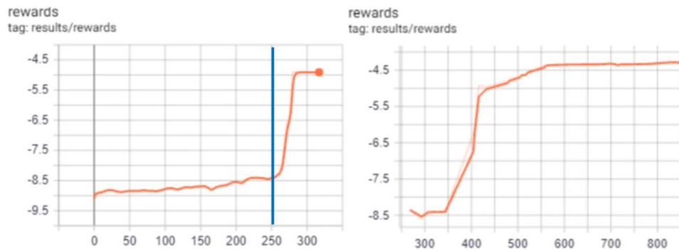
Figure 6.5: The received reward after pruning the last layer, averaged for the whole batch. From the 250 th episode, the training is continued with a smaller learning rate and higher entropy.
