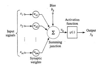
Figure 2: Nonlinear model of a neuron [20]
