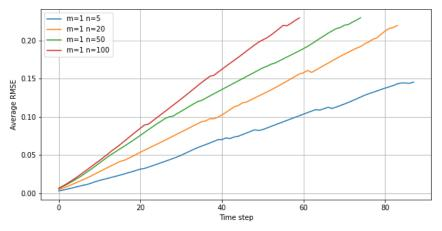
Figure 32: Change of average RMSE for Na+ parameter at different prediction lengths
