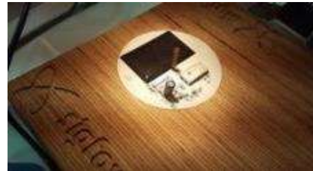
A prototype using solar energy to generate Sigfox messages
