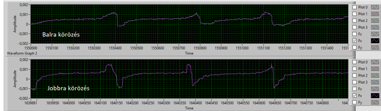
Out-of-balance voltage proportional to radial force component ( F_x )
