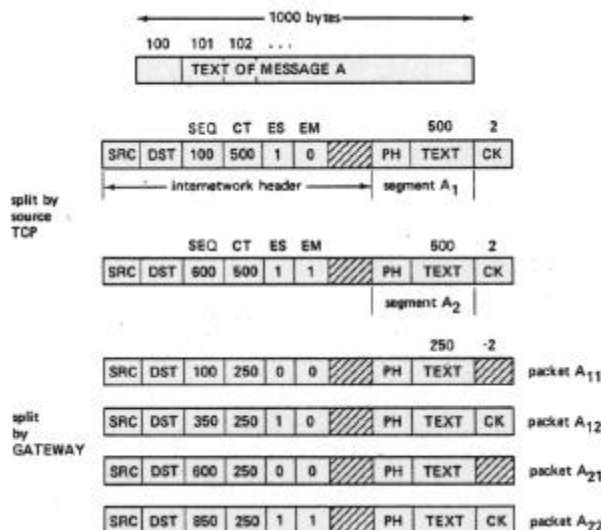
Fig. 9. Message splitting and packet splitting.
