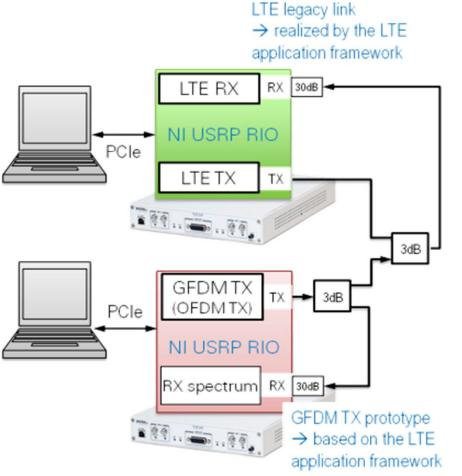
5GNOW 5G demo scenario Fragmented spectrum use case with Synchronous LTE legacy link + Asynchronous 5G user using non-orthogonal GFDM waveform Legacy LTE signal Asynchronous 5G user using GFDM /OFDM Visualization/KPIs BLER of the legacy LTE system BX OAM constellations TX + RX power spectra
