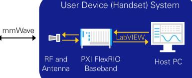
The experimental 5G PoC system will be implemented using National Instruments' baseband modules which make up the state-of-the-art system for **rapid prototyping** of 5G air interfaces today.
